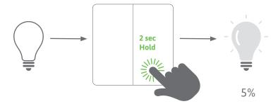
A longer press (2 seconds) on the switch when it is switched off can be used to activate the night light. The light starts at 2% brightness.
