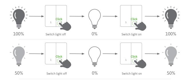
Behavior of the color mood with DUO Receiver: Here the system remembers the set color temperature in addition to the brightness.
