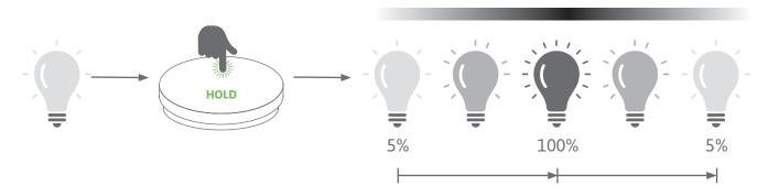
A longer press on the switch can be used to continuously increase or decrease the brightness.
