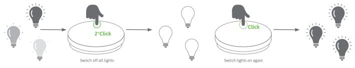
All lights are switched off. This function is used to synchronize several lights when they are running asynchronously.
