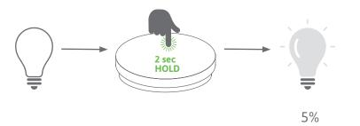
A longer press (2 seconds) on the switch when it is switched off can be used to activate the night light. The light starts at 5% brightness.
