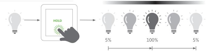
A longer press on the switch can be used to continuously increase or decrease the brightness or color temperature. This enables precise adjustment of the lighting according to individual preferences. By default, the light starts at 50% brightness or 0% cool white and 100% warm white for DUO systems. Pressing and holding the dimming function starts the light with cyclical dimming.
