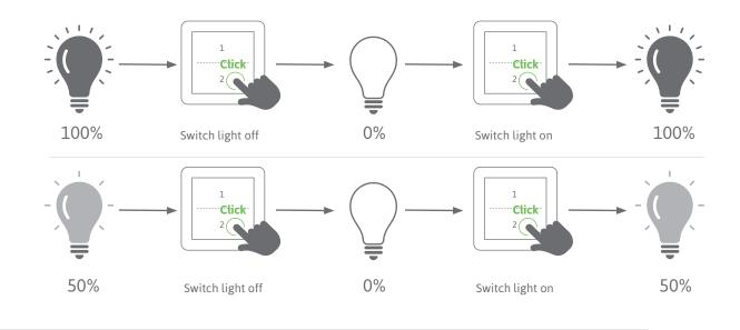
Behavior of the color mood with DUO Receiver: Here the system remembers the set color temperature in addition to the brightness.
