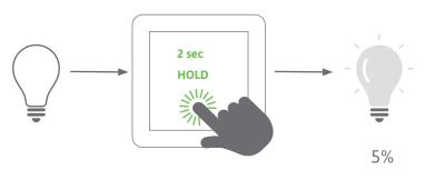
A longer press (2 seconds) on the switch when it is switched off can be used to activate the night light. The light starts at 5% brightness.
