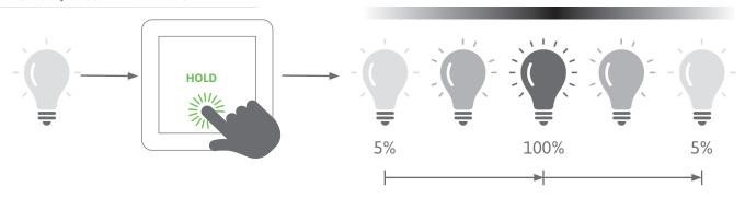
A longer press on the switch can be used to continuously increase or decrease the brightness or color temperature.
