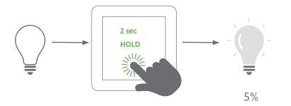
A longer press (2 seconds) on the switch when it is switched off can be used to activate the night light. The light starts at 5% brightness.
