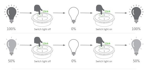
Behavior of the color mood with DUO Receiver: Here the system remembers the set color temperature in addition to the brightness.
