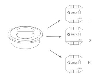
1 PushPower control unit can control any number of receivers.
