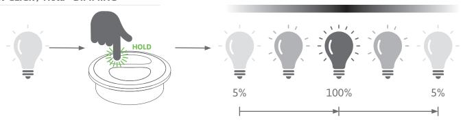
A longer press on the switch can be used to continuously increase or decrease the brightness or color temperature.
