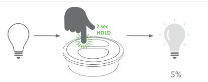
A longer press (2 seconds) on the switch when it is switched off can be used to activate the night light. The light starts at 5% brightness.
