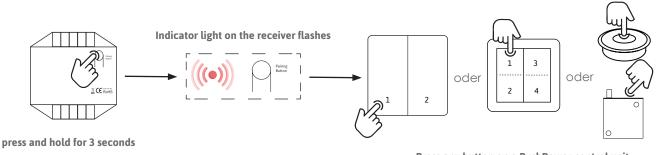
Press any button on a PushPower control unit.
