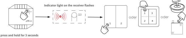
Press any button on a PushPower control unit.
