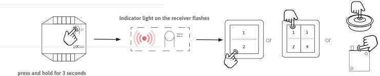
Press any button on a PushPower control unit. 2-way switch (2 options) or 4-way switch (4 options) or press the contact point for sensors
