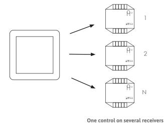
1 PushPower control unit can control any number of receivers.
